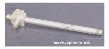
These splitters are based on Microlab Model Dx-85FN series of 2, 3, and 4 way Power Splitters. Each has been designed to evenly split high power cellular signals with minimal reflections or loss. All joints are moisture sealed to meet the IP67 rating. The design allows simple attachment to wall using the supplied bracket and clip.
